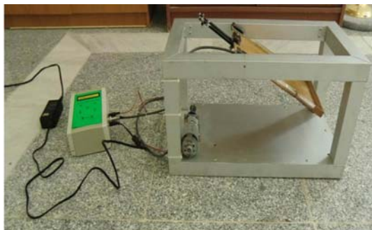
Figure 4 View of the frame, electromotor with gearbox, display box and adaptor
