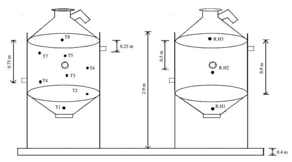
Figure 2 Temperature and relative humidity sensors' positions in the silo
