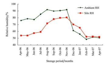
Figure 7 Relationship between the ambient relative humidity and relative humidity inside the silo with storage period
