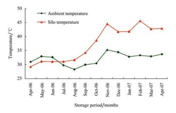
Figure 4 Relationship between the ambient temperature and the temperature inside the silo
