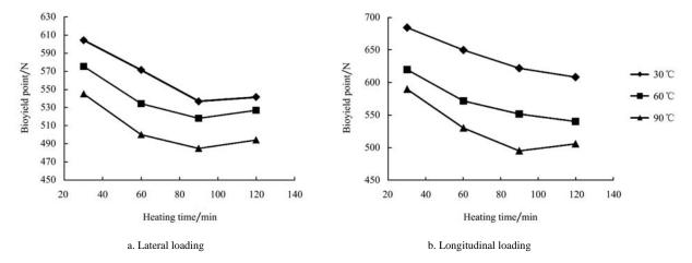
Figure 1 Variation of bioyield point of balanites aegyptiaca nut with temperature and heating time at different loading orientations
