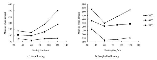
Variation of modulus of resilience of balanites aegyptiaca nut with temperature and heating time at different loading orientations
