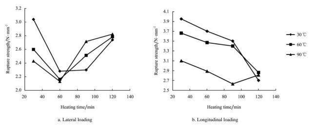
Figure 6 Effect of temperature and heating time on the rupture strength of balanites aegyptiaca nut at different loading orientations
