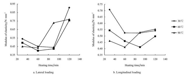
Variation of modulus of elasticity of balanites aegyptiaca nut with temperature and heating time at different loading orientations
