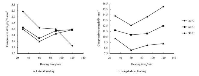
Figure 5 Effect of temperature and heating time on the compressive strength of balanites aegyptiaca nut at different loading orientations
