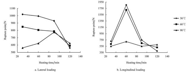
Figure 3 Variation of rupture point of balanites aegyptiaca nut with temperature and heating time at different loading orientations
