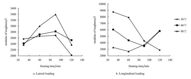
Figure 10 Variation of modulus of toughness balanites aegyptiaca nut with temperature and heating time at different loading orientations
