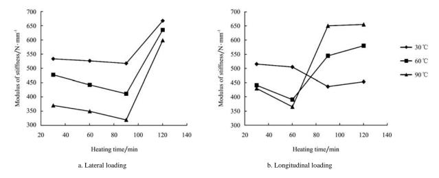
Variation of modulus of stiffness of balanites aegyptiaca nut with temperature and heating time at different loading orientations
