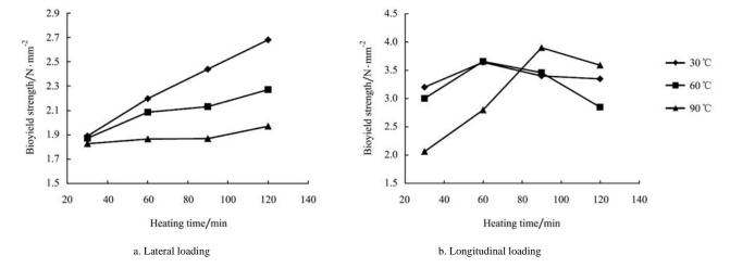
Figure 4 Effect of temperature and heating time on the bioyield strength of balanites aegyptiaca nut at different loading orientations
