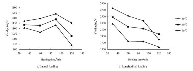
Figure 2 Variation of yield point of balanites aegyptiaca nut with temperature and heating time at different loading orientations
