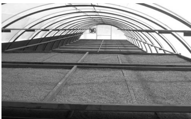
Figure 5 Inside view of solar tunnel dryer during loading
