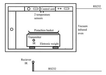
Figure 2 Schematic diagram of laboratory vacuum-infrared dryer
