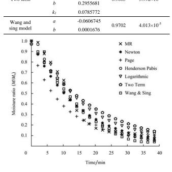
Figure 5 Variation of moisture ratios from different drying models versus drying time for Khany pistachios samples in vacuum drying process
