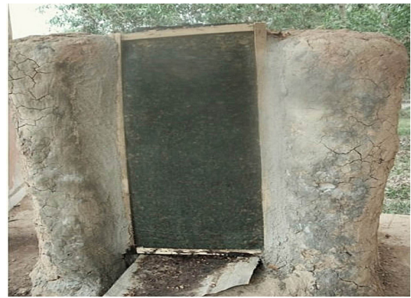
Figure 2 A prototype developed mud (Clay) evaporative cooler
