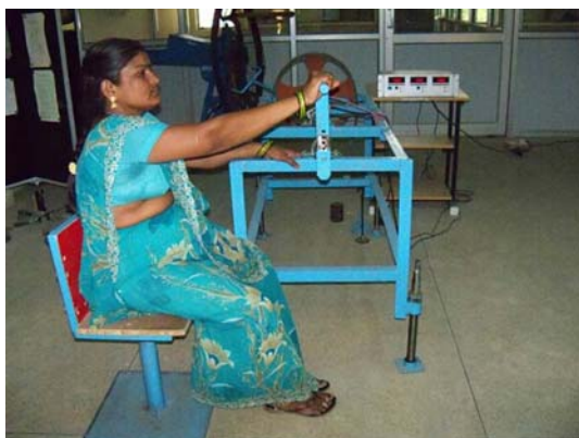
Figure 2 Force exerted by farm woman in standing and sitting postures at top positions of handle
