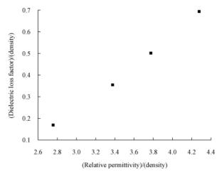
Figure 5a Dependance of (Dielectric loss factor)/(density) as a function of (Relative permittivity)/(density)corresponding to experimental complex permittivity data of soybeans at 2.45 GHz and 24°C
