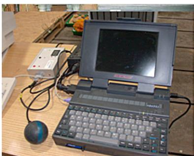
Figure 2.1 Pressure Measuring Sphere PMS-60 to measure fruit impact forces on-line
