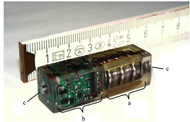
Note: a = battery, b = electronic circuitry with acceleration sensor, data processor, and data transmitter, and c = contact points for recharging
