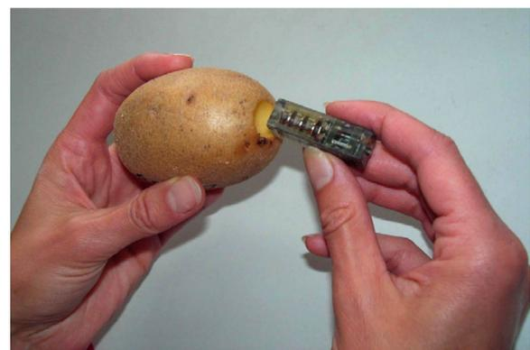
Figure 3.2 Implantation of the AMU into a potato tuber.
