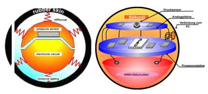
Figure 2.3 Internal electronic units of the PMS-60.
