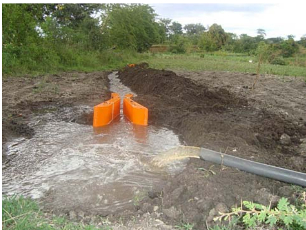
Plate 2 Water flow measurement using a Parshall flume in a sub canal
