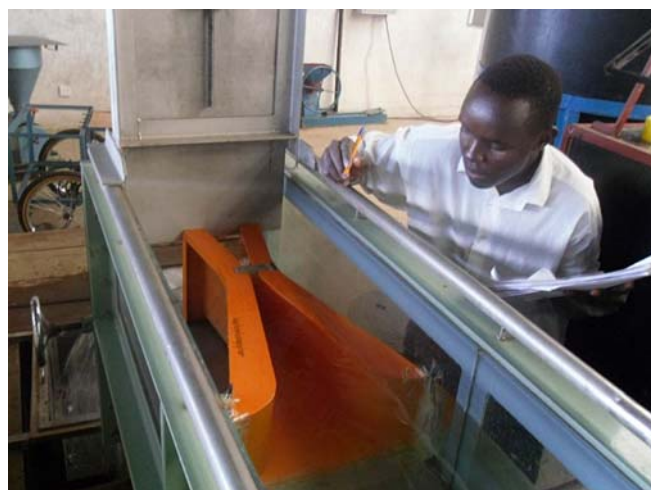
Plate 1 Calibration process for the Parshall flume
