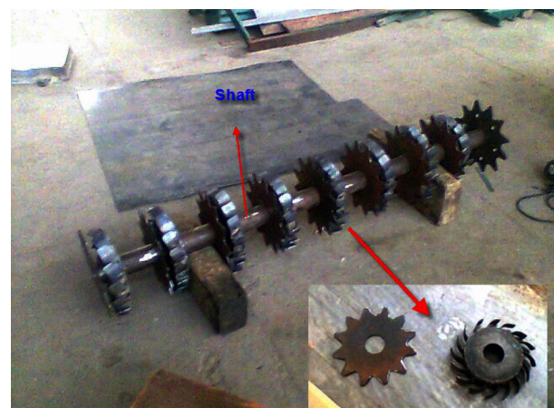
Figure 3 Arrangement of the residue manager parts on its shaft
