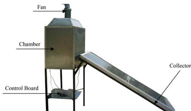
Figure 1 Experimental forced convection solar dryer
