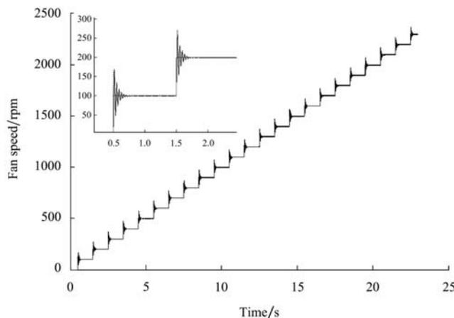
Figure 7 Simulated model responses to different speeds
