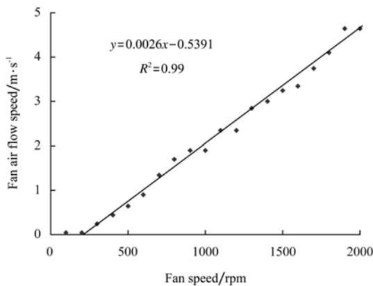
Figure 2 Variation of the fan outlet air speed with the fan speed
