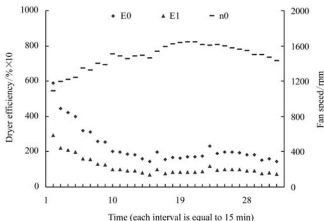
Figure 8 Efficiency and controlled fan speed variations with time
