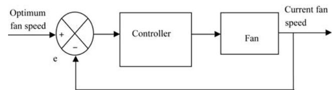
Figure 3 Block diagram of fan speed control system
