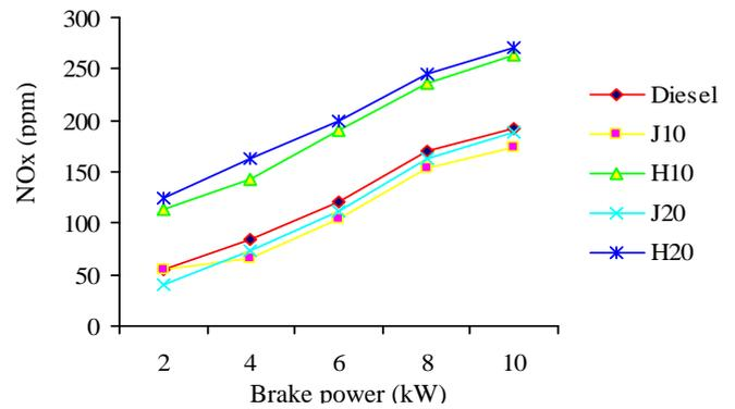
Figure 7 Variation of NO<sub>x</sub> emission with load
