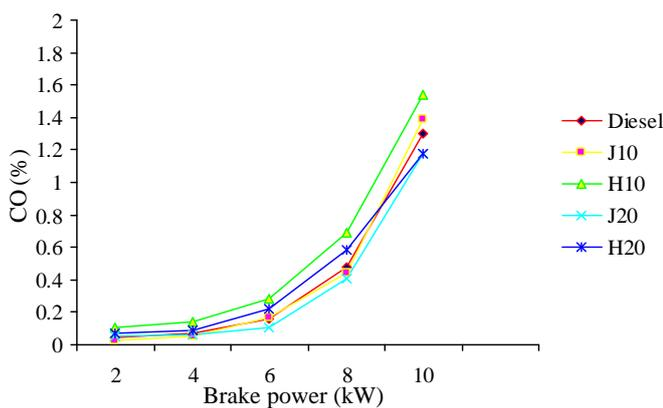
Figure 6 Variation of CO emission with load
