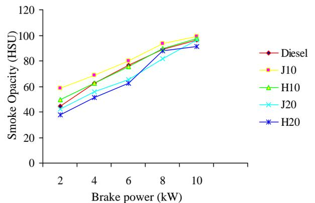
Figure 8 Variation of smoke emission with load
