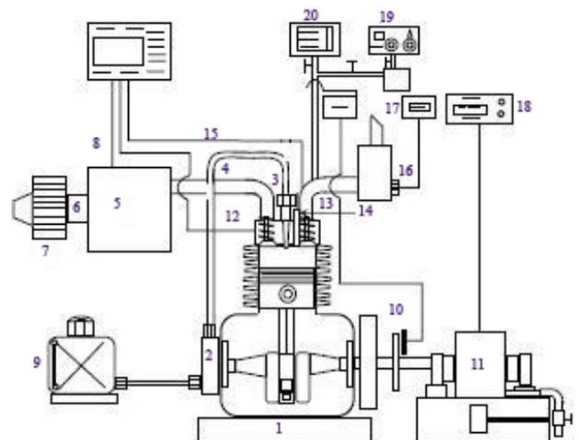
1. Engine 2. Fuel injection pump 3. Fuel injection nozzle 4. Intake manifold 5. Intake air surge tank 6. Air flow meter 7. Air cleaner 8. Intake air temp sensor 9. Fuel tank 10. Crank angle detector 11. Electric dynamometer 12. Coolant temp sensor 13. Exhaust manifold 14. Compression pressure transducer 15. Exhaust gas temp sensor 16. Air-fuel ratio sensor 17. A/F meter 18. Dynamometer control panel 19. Gas analyzer 20. Smoke meter
