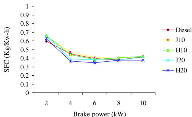
Figure 4 Variation of specific fuel consumption with load
