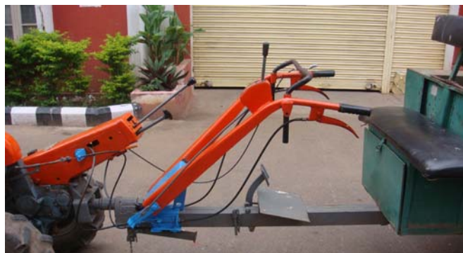
Figure 1 7 hp diesel walking tractor with removed handles from body and rigidly fitted in front of the toe bar of the trailer with a bracket
