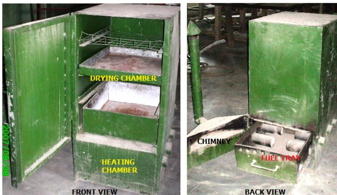
Figure 1. The biomass furnace-dryer: drying chamber and the fuel compartment.
