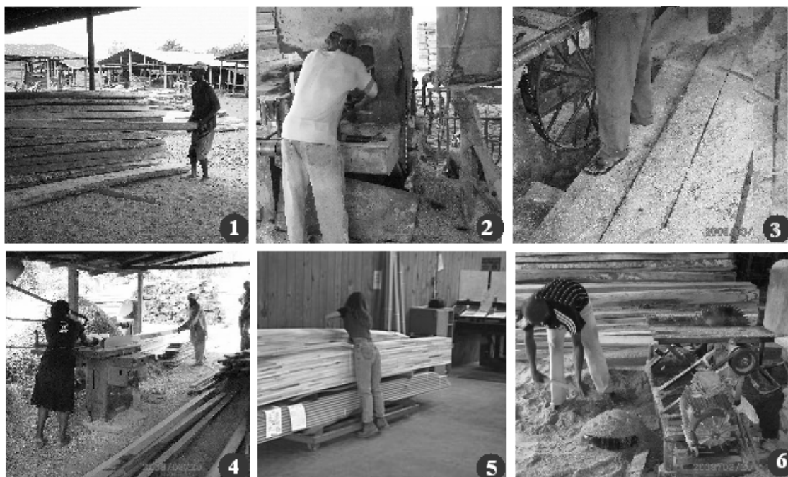
Figure 1 Identifiable hazards in sawmill sites: 1) Manual Lifting and stacking sawn lumber, 2& 3) Non-use of protective wears and equipment during maintenance, 4 & 5) Repetitive motion, twisting and reaching for objects and 6) Breathing in of noxious or toxic chemical emissions during waste disposal with head pan
