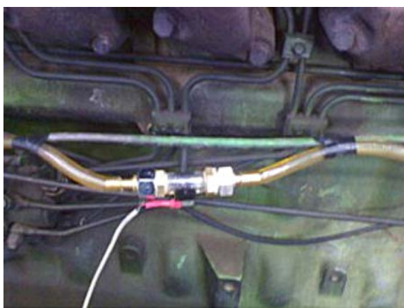
Figure 5 A view of a flow meter in contact with the engine to study the effects of vibration
