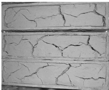
Figure 13 Shrinkage and cracks for clay samples
