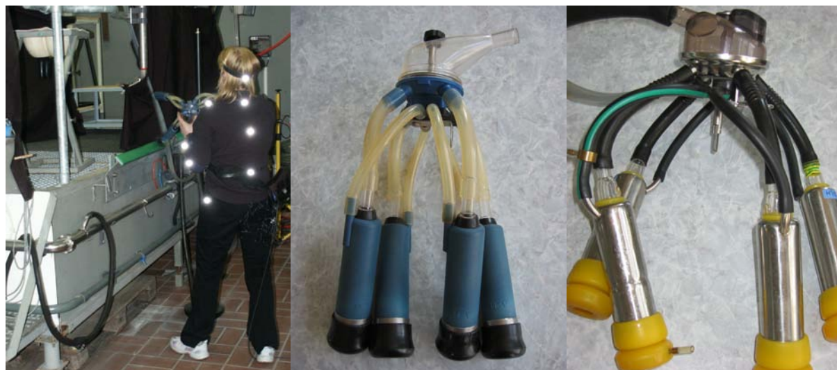
Figure 1: Experimental setting working height above shoulder level using the light milking unit (photo in the middle) showing the marker positions
