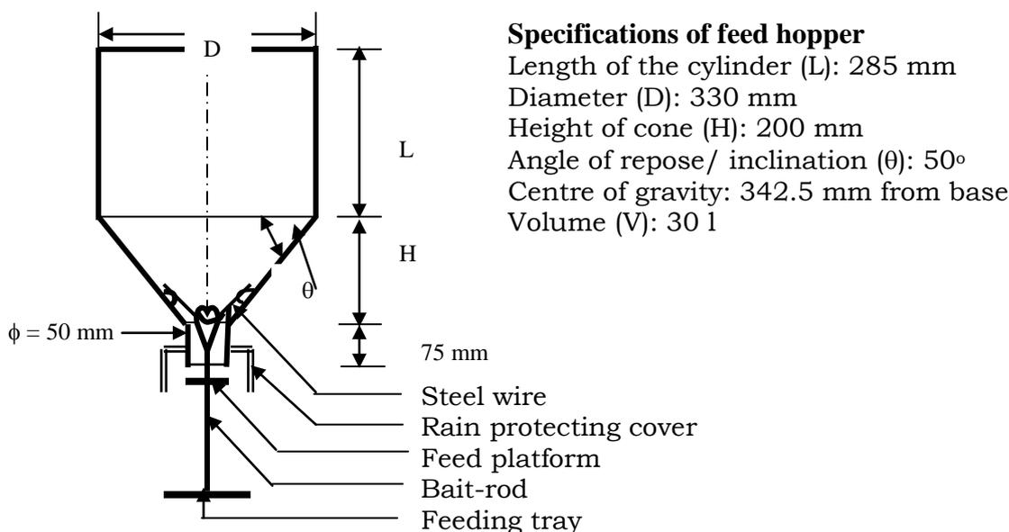
**Fig.1. Schematic diagram of FRP demand feeder hopper**
