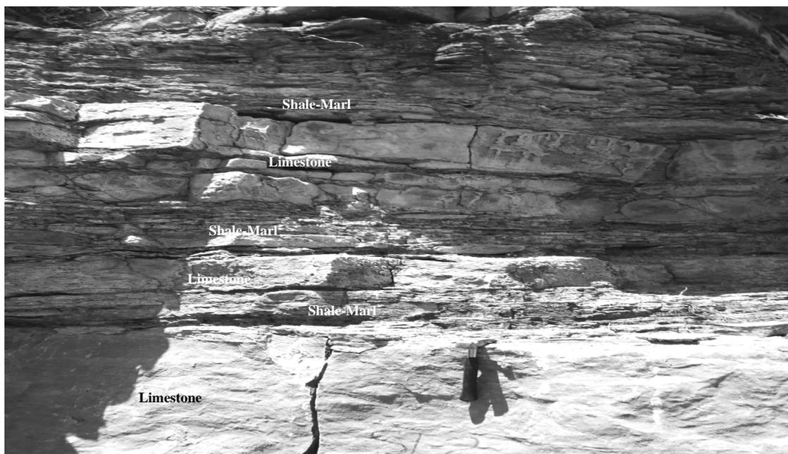
Figure 4 Limestone-shale-marl intercalation unit exposed on the left reservoir side
