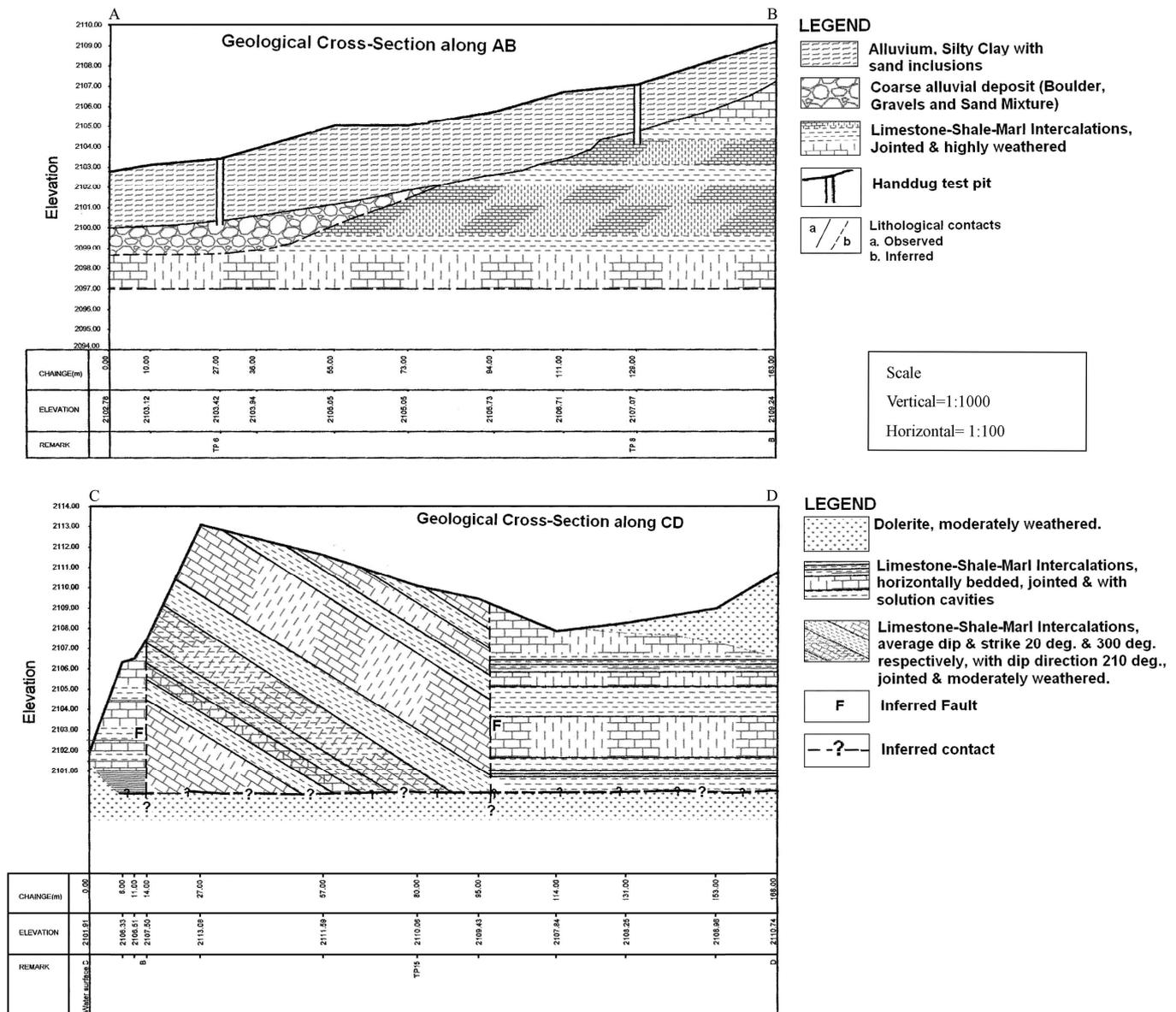
Figure 15 Engineering geological cross-section along AB and CD
