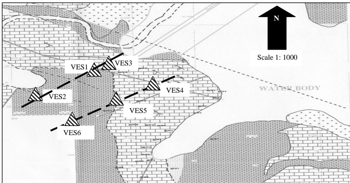
Figure 9 Location of vertical electrical sounding (VES) points
