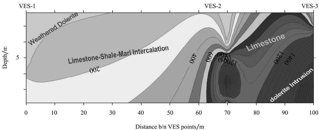
Figure 11 Geo-electrical-section (Ohm-meters) along VES1, VES2 and VES3
