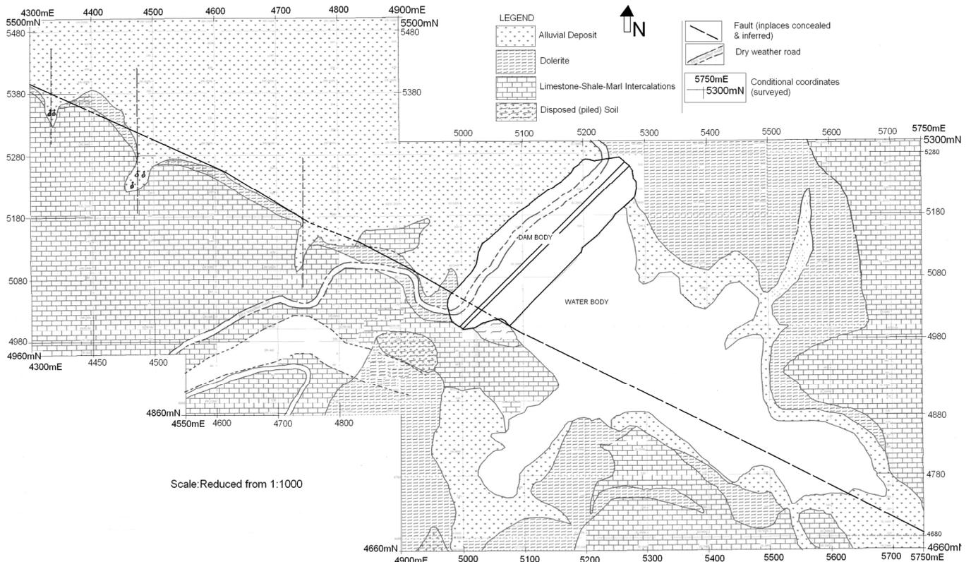
Figure 3 Geological map of Hashenge dam site and its reservoir area
