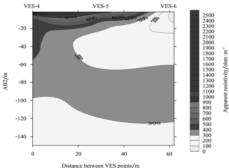
Figure 12 Apparent resistivity pseudosection (Ohm-meters) along VES4, VES5 and VES6
