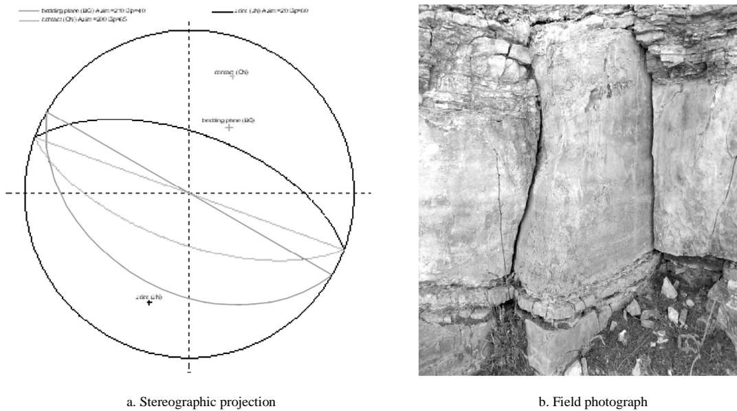
Figure 8 Bedding and tectonic joints
