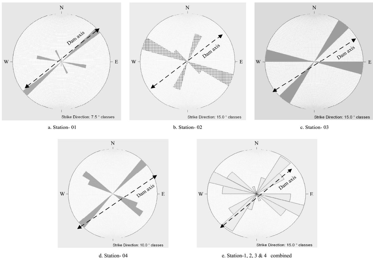
Figure 7 Stereogram of discontinuities (left abutment), double arrow shows dam axis orientation
