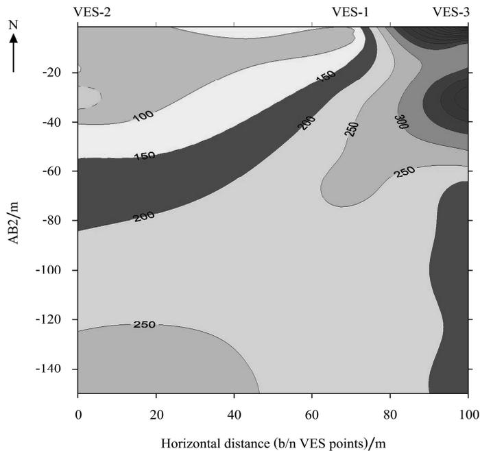
Figure 10 Apparent resistivity pseudosection (Ohm-meters) along VES2, VES1 and VES3
