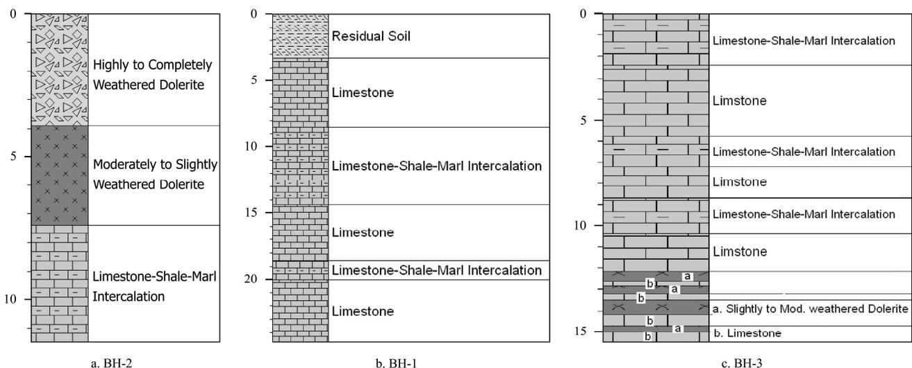
Figure 16 Simplified lithological log of the three boreholes
