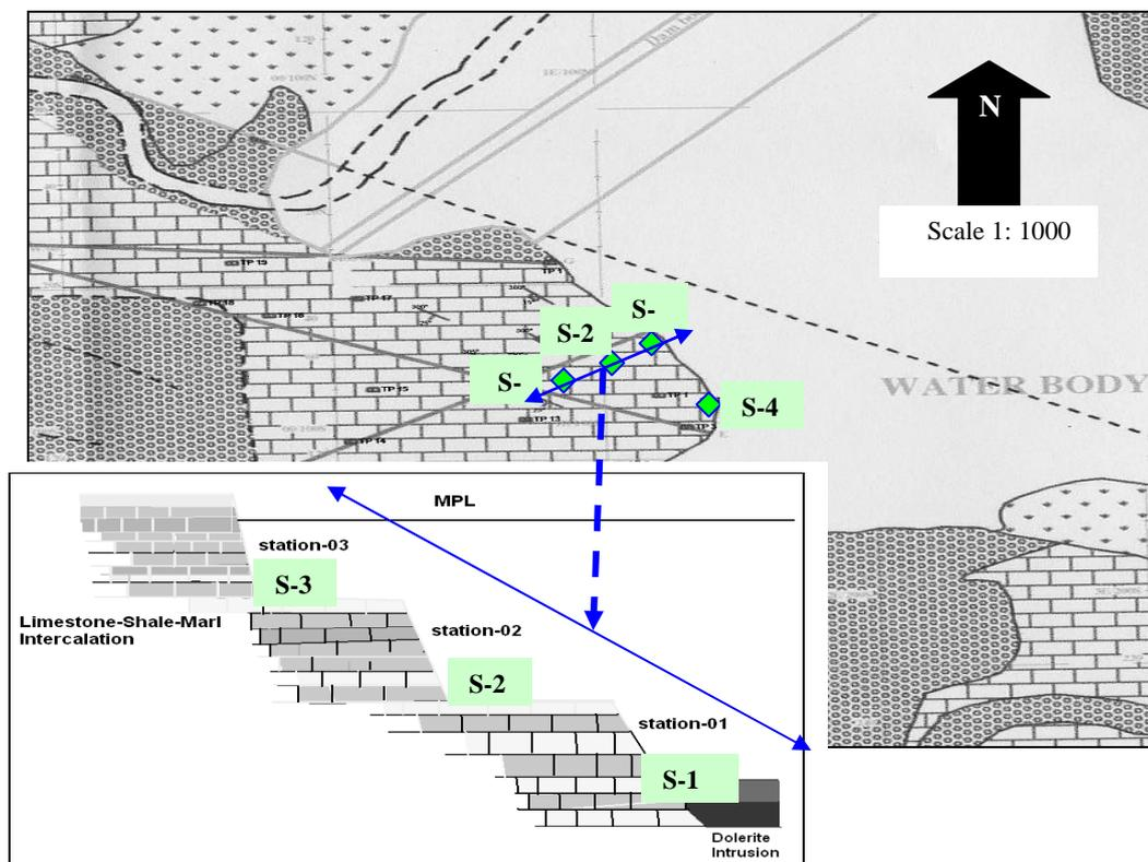
Figure 5 Simplified location of map of station points for discontinuity measurement
