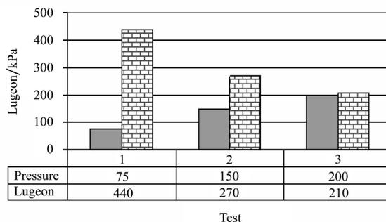
Figure 17 Bar chart showing relationship of test pressure and Lugeon value
