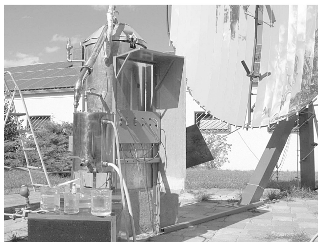
Figure 2 Solar distillation system for essential oils extraction using Scheffler reflector
