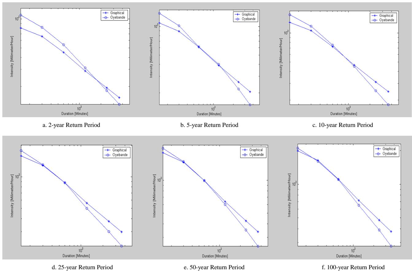
Figure 8 IDF curves obtained by the graphical method and Oyebande (1983) for Enugu location
