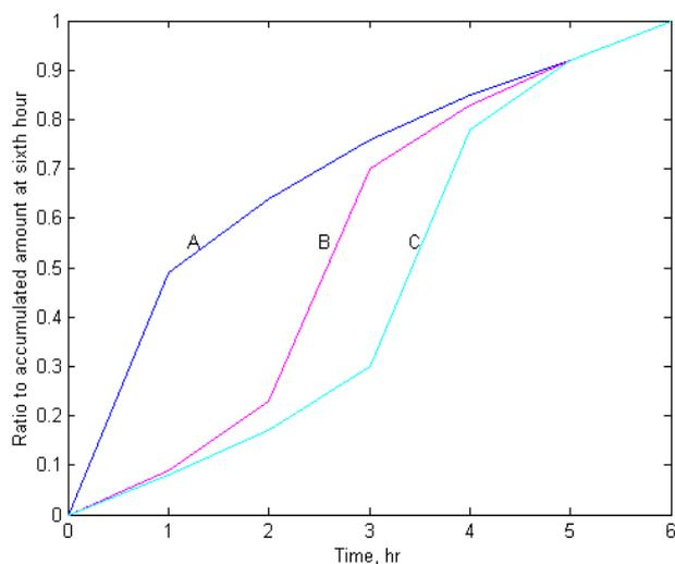
Figure 4 Generalized accumulated rainfall curves for A (advanced), B (intermediate), and C (retarded) types of storms. (USDA SCS, 1955)
