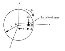
Figure 2 Schematic diagram of the motion of a particle on a slotted disc
