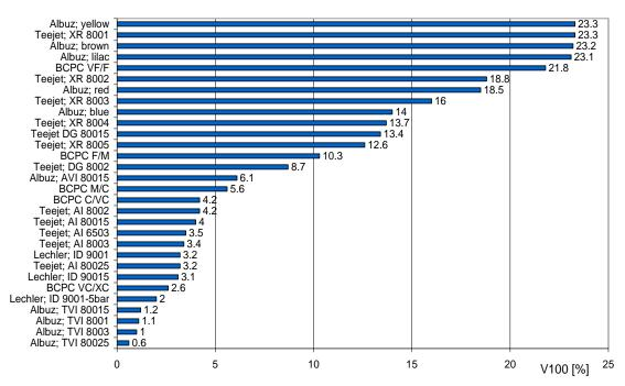
Figure 2. Ranking of measured nozzles used in orchard spraying based on volume of drops smaller than 100  $\mu$ m (V<sub>100</sub>)
