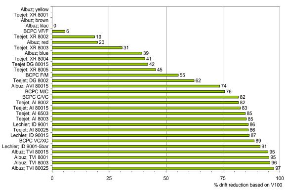
Figure 3. Potential in spray drift reduction based on  $V_{100}$  (DR<sub>V100</sub>) relative to the reference nozzle Albuz Lilac (7 bar spray pressure)
