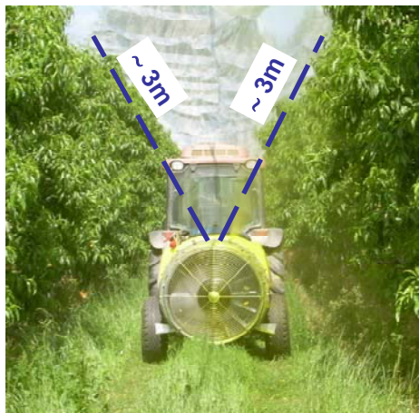
Figure 1. Example of typical orchard spray application carried out with an axial fan air-assisted sprayer: the distance between nozzles and top of trees is underlined.
