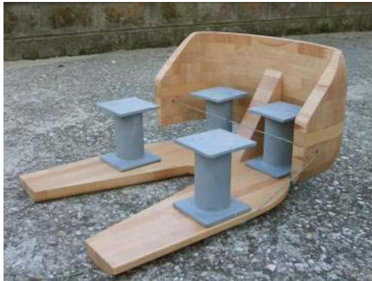
Figure 3. Device for SIP determination, completed with steels pedestals to support the ballasting.
