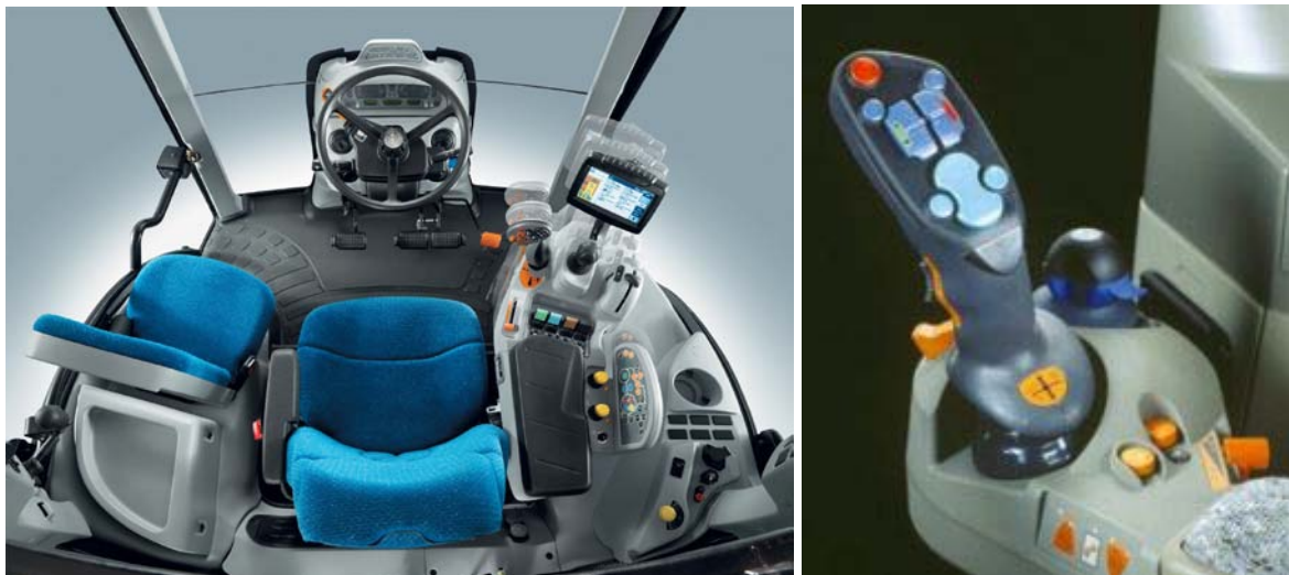
Figure 1. View of a modern tractor cab (left - NH tractor) and detail of the joystick for controlling the vehicle mobility (right – Fendt tractor).
