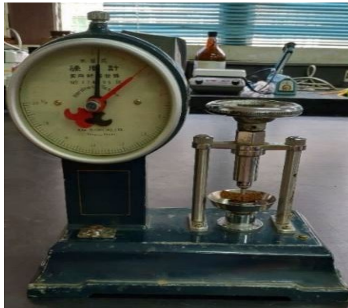
Figure 6 Hardness testing of produced sugarcane tops based pelleted feeds
