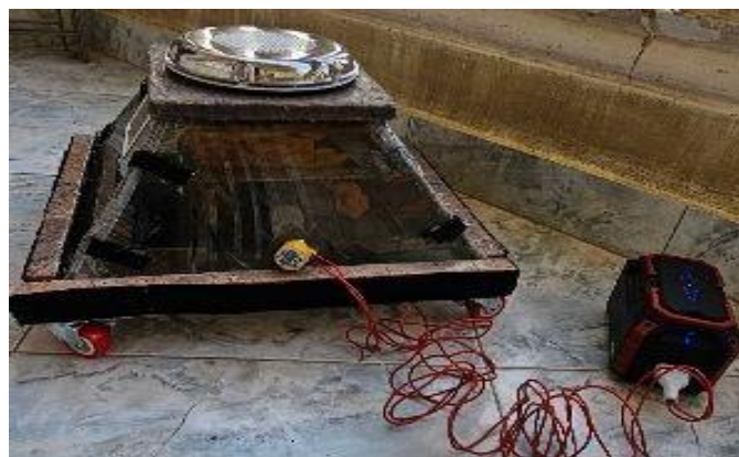
Figure 2 The portable solar dehydrator with the solar fan and the generator.
