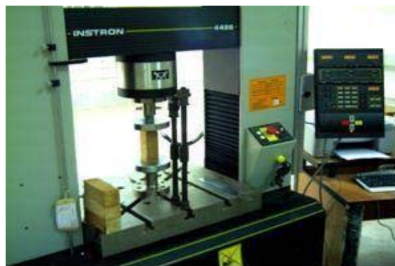
Fig.3. Compressive strength test parallel to trunk fibers
