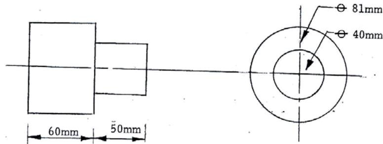
Figure 5. Front and end views of piston showing its dimension
