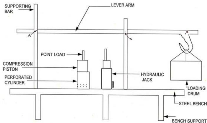
Fig. 1. Schematic diagram of the laboratory press
