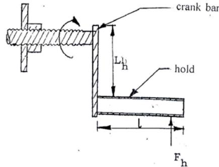
Figure 4. A section through the turning handle assembly
