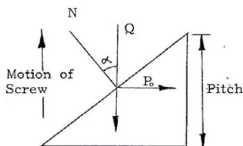
Figure 3. The vector solution of force  $P_o$  required for overcoming load  $Q$  neglecting friction
