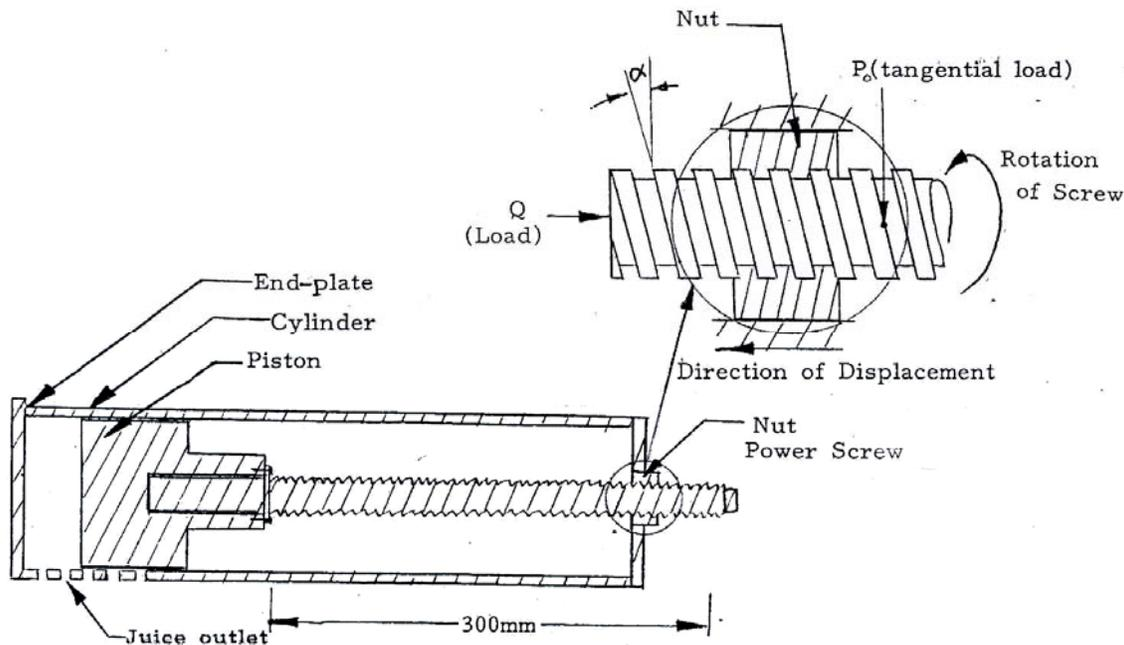
Figure 2. A section through the power screw/cylinder assembly showing the forces acting on the power screw
