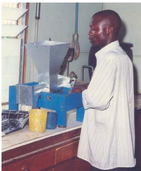
Figure 7. A view of the cashew juice extractor during testing
