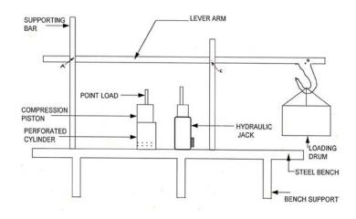
Fig. 1. Schematic diagram of the laboratory press (Ajibola *et al.*, 2000, Ajibola *et al.*, 2002).
