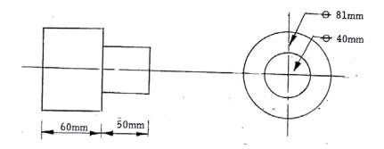
Figure 5. Front and end views of piston showing its dimension
