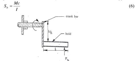
Figure 4. A section through the turning handle assembly
