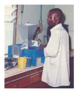
Figure 7. A view of the cashew juice extractor during testing
