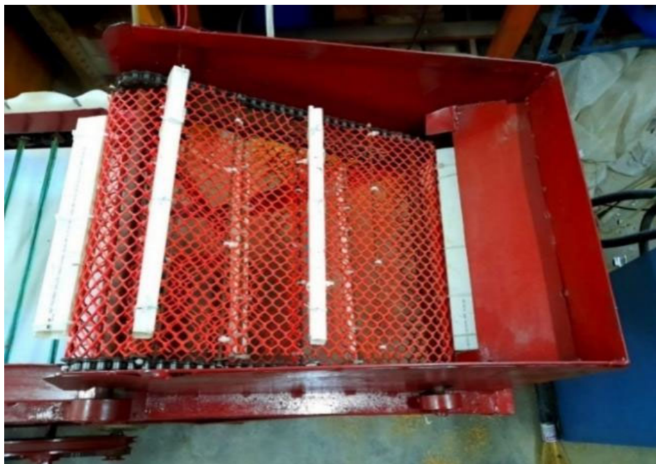
Figure 4 Tomato lifting system
