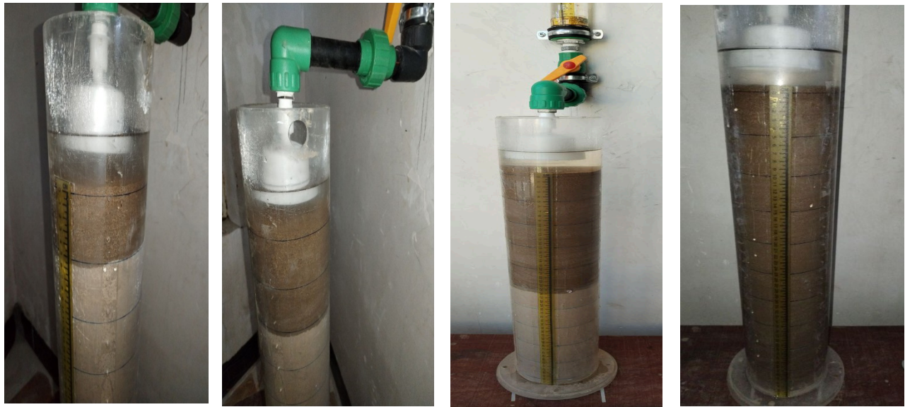
Figure 2 Wetting front progress
