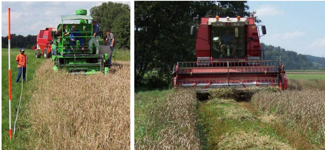
Figure 1. The plot combine was followed by a commercial combine with two yield monitors and a wider head, which also picked up the straw left behind by the plot combine.
