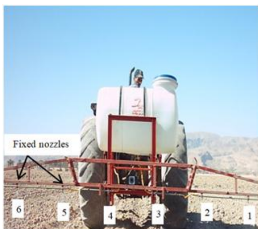
Figure 2 Band sprayer boom with fixed nozzles
