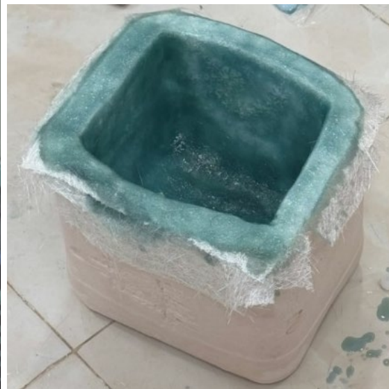
(a) Outer frame manufactured by 3D printer, (b) tank manufactured manually
