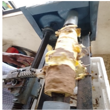
Plate 2: Peeling operation on the yam peeling machine
