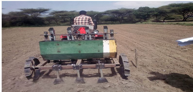
Figure 4 Garlic Clove Planter under Operation
