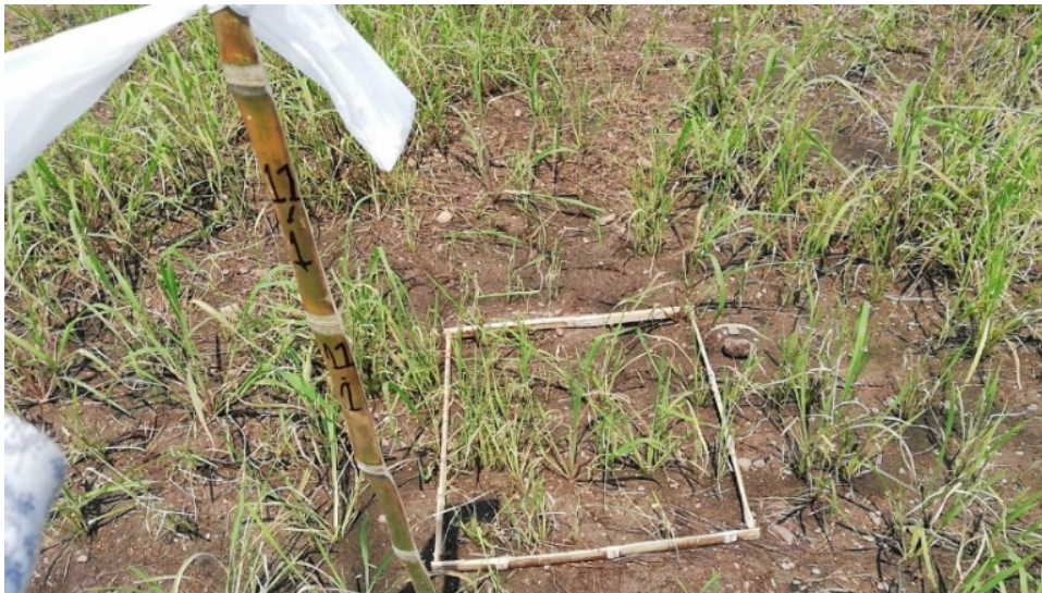
Figure 3 Gauge frame located at sampling point
