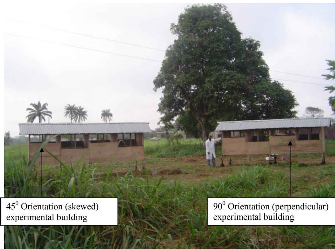
Figure1 Experimental building set-up showing both the (i) Perpendicular [ $90^{\circ}$ ] and Skewed [ $45^{\circ}$ ] orientations to the direction of the prevailing wind
