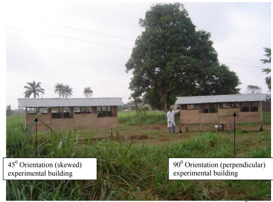
Figure 1 Experimental building set-up showing both the (i) Perpendicular [90<sup>0</sup>] and Skewed [45<sup>0</sup>] orientations to the direction of the prevailing wind
