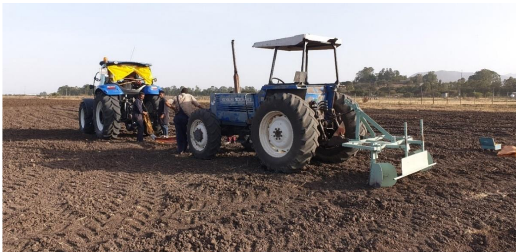
Figure 5 Measurement of the draft of the broad-bed maker using a dynamometer
