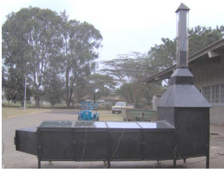
Figure 1: Solar tunnel dryer
