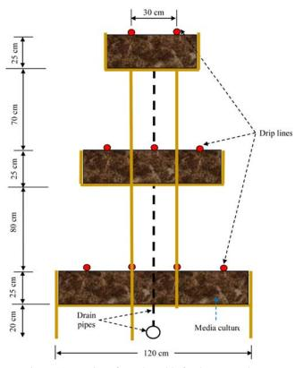
Figure 11 Design of wooden table for three green layers
