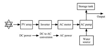
Figure 1 A schematic diagram of the water pumping system using PV energy
