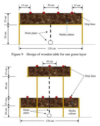
Figure 10 Design of wooden table for two green layers
