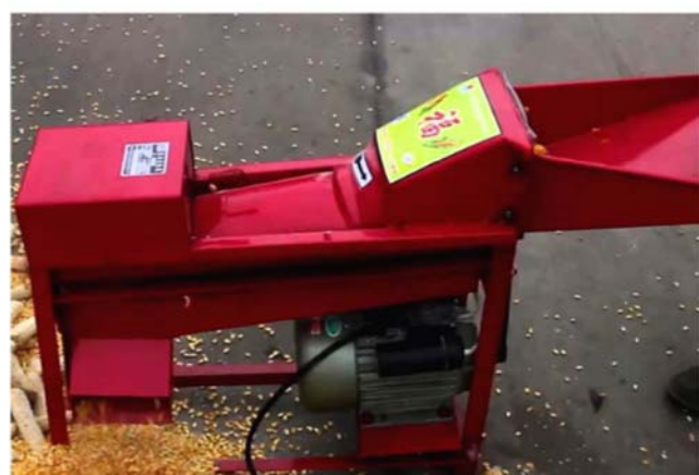
Figure 2 Machine (type MGI-TY 60) used for thresher maize
