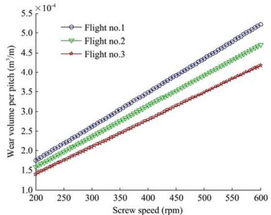
Figure 7 Relationship between the screw speed and wear volume of the screw extruder biomass briquetting machine for the first three flights from the briquetting die.
