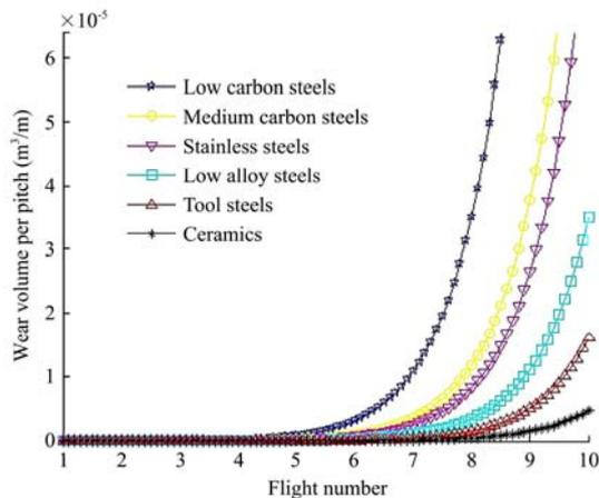
Figure 8 Influence of material of screw on the worn volume of the screw of a biomass briquetting machine
