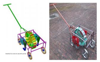
Figure 1 Isometric and photographic view of the applicator
