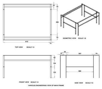
Figure 6 Different views of the frame of the applicator
