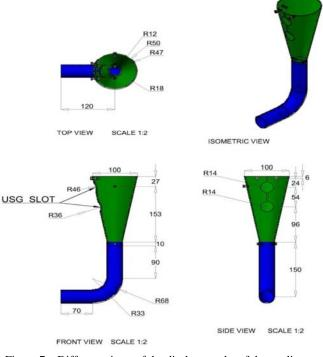
Figure 7 Different views of the discharge tube of the applicator
