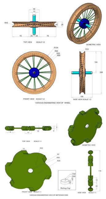
Figure 3 Different views of the drive 1heel and metering disk
