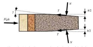
Figure 2 Mechanism to regulate the density of the bale
