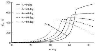
Figure 7 Operating force  $F_{op}$  versus the lever angle  $\alpha$ , for different initial values  $\alpha_o$
