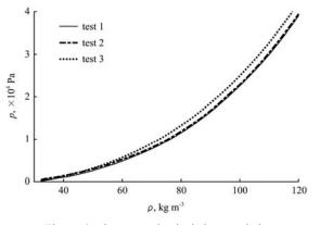
Figure 6 Straw mechanical characteristic
