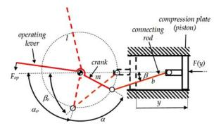
Figure 4 Baler slider-crank mechanism. Initial position (hatched line); generic position (continuous line)
