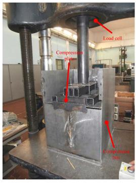
Figure 5 Straw mechanical characterisation setup
