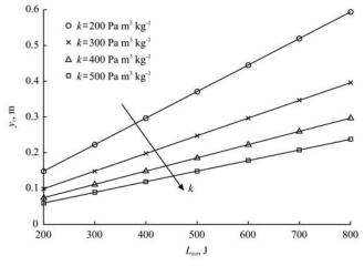
Figure 3 Piston stroke  $y_c$  per cycle related to the total work for each cycle  $L_{tot}$  (straw stiffness constant k,  $m_{tot} = 17.5$  kg,  $\rho_o = 30$  kg m<sup>-3</sup>,  $\rho_f = 120$  kg m<sup>-3</sup>)
