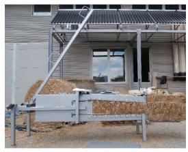
Figure 11 The prototype of the Anpilpay 2.0 press
