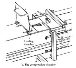
Figure 9 Details of the density regulation system and of the compression chamber
